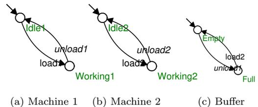
Fig. 2. Models for the two machines and the buffer.
